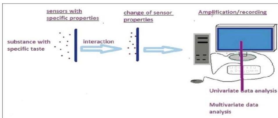
Fig 5 : Basic principle of electronic taste sending system[16]
