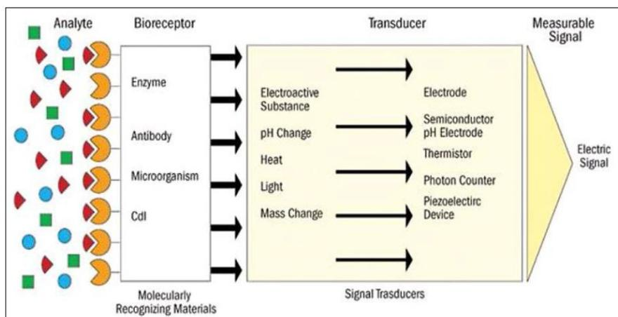
Fig 2: Biosensors and its parts.
